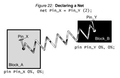
If the spring is relatively weak, as it is in Figure 22, the spring stretches easily. Consequently, Block\_A and Block\_B are placed in the general vicinity of each other, but not necessarily closely together. By increasing the strength or weight on the net, the blocks are pulled closer together, as illustrated in Figure 23. Increasing the net weight from 2 to 500 strengthens the connection between the blocks, pulling them closer together.
