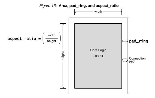
The Silistix software uses the values specified by the designer when calculating the percentage of total die area utilized by the interconnect logic. These values are used by the First Placement Estimator (FPE) tool for floor planning purposes. The area specified for the entire system takes precedence over the calculated value from the area values set for each endpoint when determining total area. However, the area values set for the endpoints are still used by the FPE tool.
