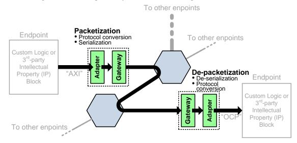
Figure 9: Switching Latency is Total Network Flight Time in a Direction
