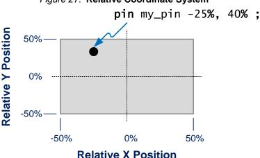
Figure 27: Relative Coordinate System
